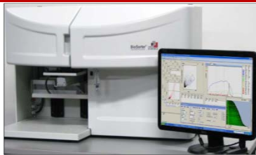
Figure 1: BioSorter ® analyzes and sorts cell clusters and large cells (10–1500 \mu\text{m} diameter) in a continuous flow stream at high rate (up to 100 events/sec). The device measures object size (TOF), optical density (EXT) and multiple fluorescent markers.
